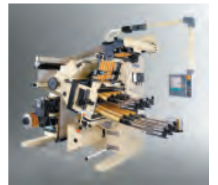
Berhalter B 500 High-performance die-cutting machine with 8-up double output punching tool Ø 75.5 mm for web width up to 520 mm
